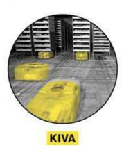
A Kiva Systems robot can scurry about the floor of a large warehouse to find ordered products. It then fetches the correct rack or pallet and brings it to a worker who packages the goods.
